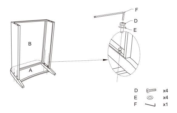
Step 2. Attach side panel (part A) to seat panel (part B) using short bolts (part D), flat washers (part E) and allen wrench (part F).
